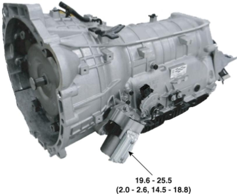
**Tightening torque : N·m (kgf·m, lb·ft)**
